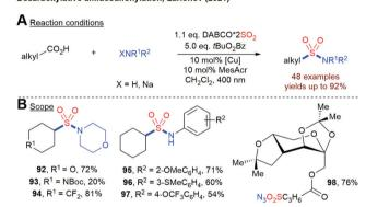
Scheme 21 Decarboxylative aminosulfonylation of free carboxylic acids using a dual catalyst system
