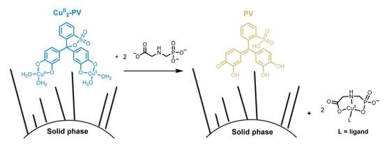
Fig. 2 Schematic representation of detection of GlyP with an immobilized Cu<sup>ll</sup>-PV complex by an indicator displacement assay using solid phase extraction.
