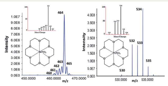
Fig. 3 Orbitrap confirmation of 18C6 [Ba-NO<sub>3</sub>] with Ba natural abundance (left) and [Pb-NO<sub>3</sub>] with Pb natural abundances (right) patterns correlating to the simulated M-L isotopic distribution.
