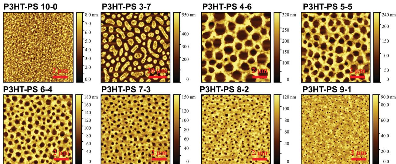
Fig. 2 AFM of the 3D structures produced from phase separation followed by acetone wash with different mixing ratios between P3HT ( $10 \text{ mg ml}^{-1}$ ) solution and added PS, given in  $\text{mg ml}^{-1}$  in chlorobenzene.
