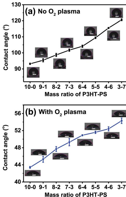
Fig. 5 Water contact angle in degrees, average  $\pm$  SD for different P3HT–PS mixing ratios, starting with neat planar 10–0 P3HT samples. As-fabricated samples (a) following leaching out of the PS, while (b) is for samples after additional treatment with  $O_2$  plasma.
