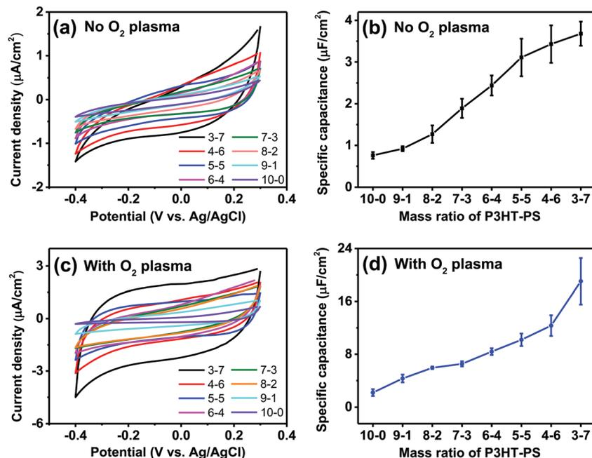
Fig. 6 Electrochemical capacitance evaluation of the structured P3HT films. (a) CV scans ( $100 \text{ mV s}^{-1}$ ) of the P3HT films in the electrochemically-passive region of P3HT. (b) Average  $\pm$  SD of capacitance in  $\mu\text{F cm}^{-2}$  for different P3HT-PS mixing ratios, versus planar. (c) CV scans ( $100 \text{ mV s}^{-1}$ ) of the  $\text{O}_2$  plasma-treated P3HT. (d) Calculated capacitance values for plasma-treated samples.
