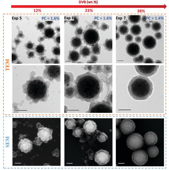
Fig. 5 TEM and SEM micrographs of PDMAEMA@MLPs synthesized by seeded semi-batch emulsion polymerization of styrene (PCtheo = 2.5%) in the presence of increasing amounts of DVB: 12 wt%, 23 wt% and 38 wt% (based on overall monomer mass) (Exp. 5, 6 and 7, respectively, Table 1), introduced either in the initial load or in both the initial load and the feed (see Table S3, ESI† for detailed experimental conditions). Scale bar: 100 nm. Additional micrographs are presented in the ESI.†
