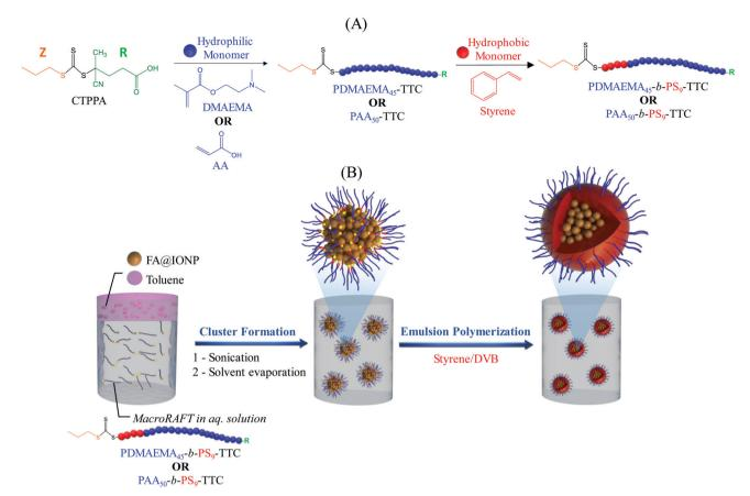
Scheme 1 Schematic representation of (A) synthesis of amphiphilic block copolymer (PDMAEMA<sub>45</sub>-b-PS<sub>9</sub>-TTC or PAA<sub>50</sub>-b-PS<sub>9</sub>-TTC), and (B) IO cluster formation via emulsification/solvent evaporation and synthesis of magnetic latex particles via emulsion polymerization using the macroRAFT-stabilized clusters as seeds.
