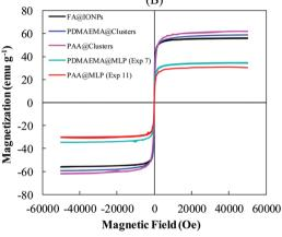
Fig. 7 (A) TGA and (B) SQUID analyses of the commercial fatty acidmodified IO nanoparticles (FA@IONPs), the PDMAEMA@clusters, the PAA@clusters, and the magnetic fraction ( $\omega_{mag}$ ) of the PDMAEMA@MLP and PAA@MLP samples (Exp. 7, Table 1 and Exp. 11, Table 2).
