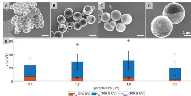
**Fig. 3** SEM pictures of Janus particles with average sizes of 0.7 μm (A), 1.2 μm (B), 1.6 μm (C), 3.5 μm (D) and their velocities (E) in 0.5% H<sub>2</sub>O<sub>2</sub> solution ( $v_m$  – mean velocity at given UV intensity,  $v_{max}$  – velocity of fastest particle), scale bar 1 μm.
