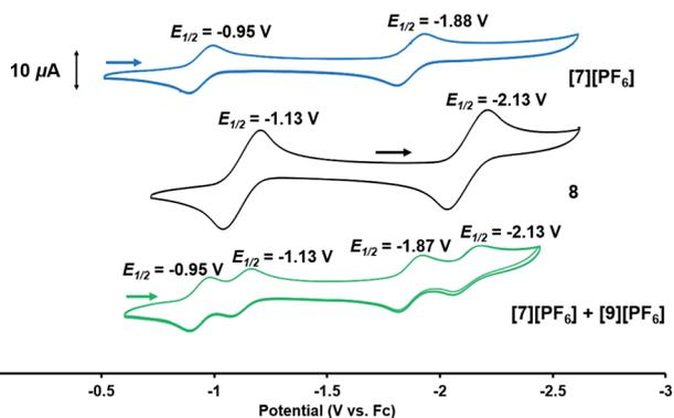
Fig. 7 Cyclic voltammograms (in 0.3 M [ $t$ Bu<sub>4</sub>N][PF<sub>6</sub>] in THF; scan rate: 100 mV s<sup>-1</sup>) of compounds [7][PF<sub>6</sub>] (blue), **8** (black), and a mixture of [7][PF<sub>6</sub>] and [9][PF<sub>6</sub>] obtained from the reaction of **8** with FcPF<sub>6</sub> (green).
