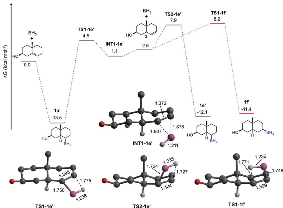
Fig. 4 Gibbs energy profiles (in kcal mol<sup>-1</sup>) for the formation of **1e'** and **1f'** and transition state structures involved. Bond distances are in Å. In the depicted structures, H atoms are omitted for clarity, except the H atom involved in the hydroboration.
