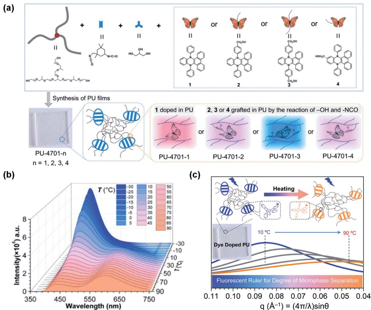
Fig. 9 (a) Diagrammatic sketch illustrating the DPAC-doped polyurethanes **PU-4701-1**–**PU-4701-4**. (b) PL spectra of **PU-4701-2** at various temperatures ( $-30$  to  $90\text{ }^{\circ}\text{C}$ ). (c) Scattering curves of **PU-4701-1** achieved by small-angle X-ray scattering at various temperatures ( $10$ – $90\text{ }^{\circ}\text{C}$ ). Reproduced from ref. 107 with permission from the American Chemical Society, Copyright 2019.
