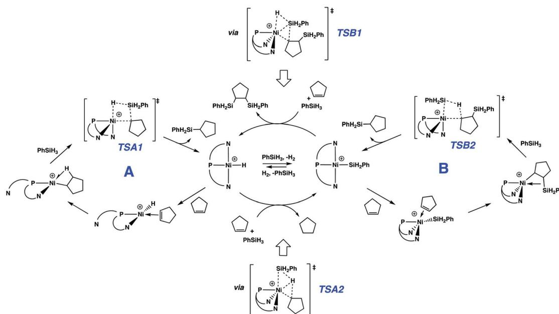
Scheme 3 Proposed mechanisms for nickel-catalyzed hydrosilation of alkenes.
