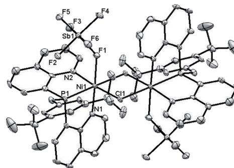
Fig. 1 ORTEP drawing of the X-ray crystal structure of **3b**. Hydrogen atoms and C<sub>6</sub>H<sub>5</sub>F are omitted for clarity. Key bond distances (Å): Ni(1)–N(1) = 2.092(6), Ni(1)–N(2) = 2.070(7), Ni(1)–P(1) = 2.347(2), Ni(1)–F(1) = 2.262(4), Sb(1)–F(1) = 1.904(4), Sb(1)–F(2) = 1.873(5), Sb(1)–F(3) = 1.877(5), Sb(1)–F(4) = 1.874(5), Sb(1)–F(5) = 1.867(5), Sb(1)–F(6) = 1.869(5).
