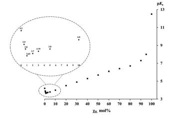
Fig. 1 p $K_a$  values of PhCH(CN)<sub>2</sub> versus the molar fractions  $\chi_{II}$  of [Bmim][NTf<sub>2</sub>] in [Bmim][NTf<sub>2</sub>]/DMSO mixtures.
