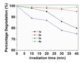
Fig. 9 Photostability of 1a-4a (1 mg/50 mL) in methanol at the absorption maximum wavelength with the irradiation time.
