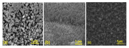
Fig. 3 SEM images of (a) undoped ZnO nanorods (b) CuO nanostructures (c) MoO<sub>3</sub> thin film.
