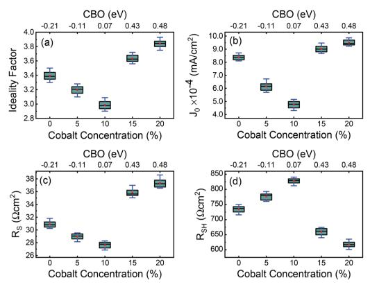
Fig. 11 Statistics of the result obtained from one diode model fitting of dark J-V characteristics of various cobalt doped ZnO layer (0–20%). (a) Ideality factor (n), (b) reverse saturation current density ( $J_0$ ), (c) series resistance ( $R_S$ ), and (d) shunt resistance ( $R_{SH}$ ). The solid red circle represents the average values, and the horizontal lines in the box denote the 25th, 50th, and 75th percentile values.
