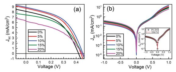
Fig. 9 (a) I-V characteristics under light and (b) dark IV characteristics of 0–20% cobalt doped ZnO/CuO heterojunction solar cells. The insets of (b) show one diode model fit of 0% ZnO/CuO solar cell.
