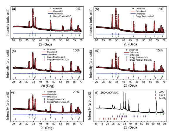
Fig. 2 XRD spectra and (a-e) Rietveld analysis of 0-20% cobalt doped ZnO nanorods (f) ZnO/CuO/MoO<sub>3</sub> heterojunction solar cell.
