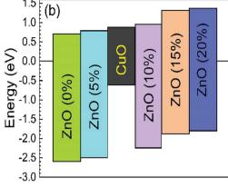
Fig. 7 (a) Band diagram of 0% cobalt doped ZnO/CuO heterojunction solar cells. (b) Schematic band offsets in 0-20% cobalt doped ZnO/CuO heterojunction. VBM and CBM values are from the Fermi level.
