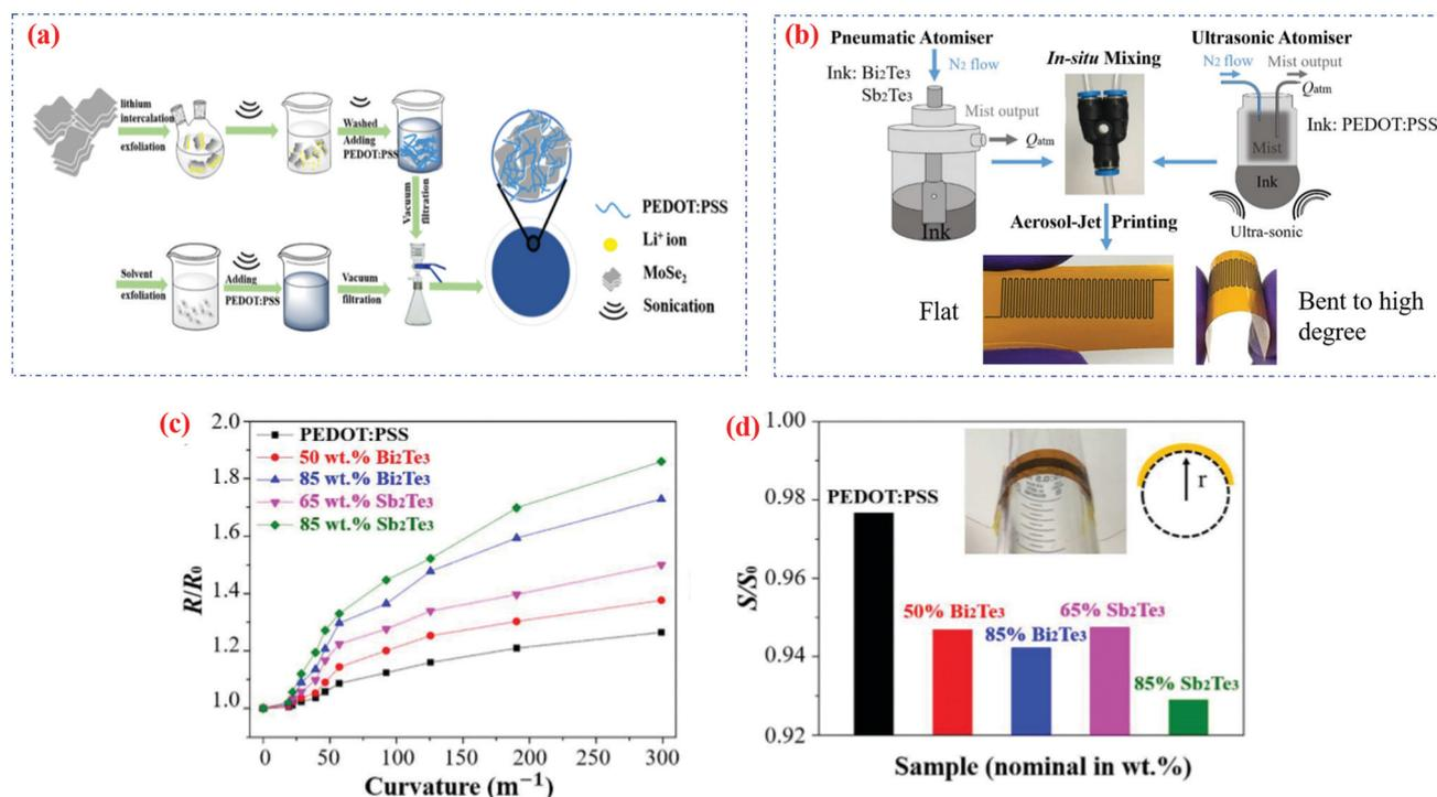
Fig. 6 (a) Schematic illustration of the preparation of the MoSe<sub>2</sub>/PEDOT:PSS composite; (b) schematic of the *in situ* mixing and aerosol jet printing method; (c and d) flexing test of printed Bi<sub>2</sub>Te<sub>3</sub> and Sb<sub>2</sub>Te<sub>3</sub>/PEDOT:PSS nanocomposites. Produced with permission.<sup>100</sup> Copyright © 2017 IOP Publishing Ltd.<sup>156</sup> Copyright © 2018 American Chemical Society.
