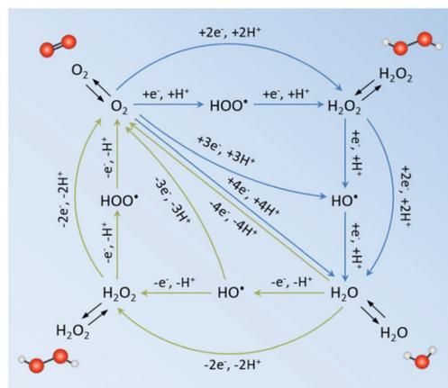
Fig. 2 Possible reduction pathways from O<sub>2</sub> to H<sub>2</sub>O (blue) and oxidation pathways from H<sub>2</sub>O to O<sub>2</sub> (green). The black arrows denote the adsorption and desorption/diffusion of species from the bulk solution and the catalyst. Oxygen and hydrogen atoms are represented as red and white balls, respectively. Stoichiometric H<sub>2</sub>O is omitted for clarity.<sup>28</sup>
