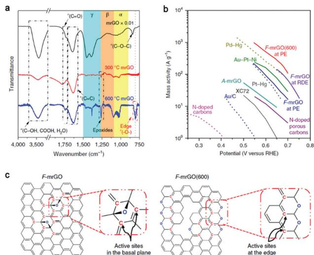
**Fig. 6** (a) FTIR spectra of various mrGO powder samples. (b) Mass activity of different electrocatalysts for  $\text{H}_2\text{O}_2$  production. The data presented as dashed lines was measured in acidic conditions (0.1 M  $\text{HClO}_4$ ) and that as solid lines was measured in basic conditions (0.1 M  $\text{KOH}$ ). (c) Idealized schemes of proposed low-overpotential active sites on F-mrGO and F-mrGO (600). Reproduced with permission.<sup>34</sup> Copyright 2018 Springer Nature.
