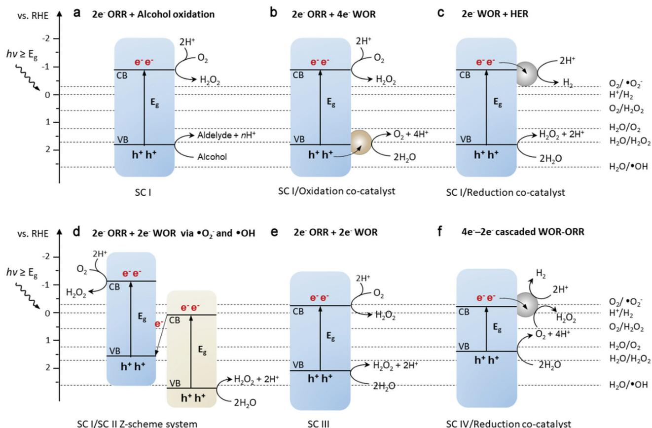
Fig. 5 Different redox pathways for photochemical  $\text{H}_2\text{O}_2$  formation (a–f) and selected redox reaction potentials regarding the oxygen reduction reaction (ORR) and water oxidation reaction (WOR). SC and HER are abbreviations of semiconductor and hydrogen evolution reaction, respectively. SCs I–IV are different semiconductors in previously reported specific systems for the photocatalytic synthesis of  $\text{H}_2\text{O}_2$ .
