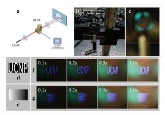
Fig. 4 (a) Schematic of the computer-controlled scanning system that employs AOD and an optical lens to control light deflection and focus. (b) Photograph of the display system. (c) The letters "UCNP" displayed on the PVA film. (d) The "UCNP" pattern and (e) grayscale gradient pattern entered by a computer. (f) "UCNP" pattern photographs and (g) greyscale gradient photographs taken at different exposure times (0.1, 0.2, 0.5, and 1.0 s).
