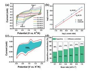
Fig. 5 (a) CV curves of NiS<sub>2</sub>/3DGO at scan rates range from 0.1 to 1.0 mV s<sup>-1</sup>. (b) Linear relationship of log(i) vs. log(v). The contribution ratio of the capacitive capacities and diffusion-limited capacities at 1 mV s<sup>-1</sup> (c) and at different scan rates (d).
