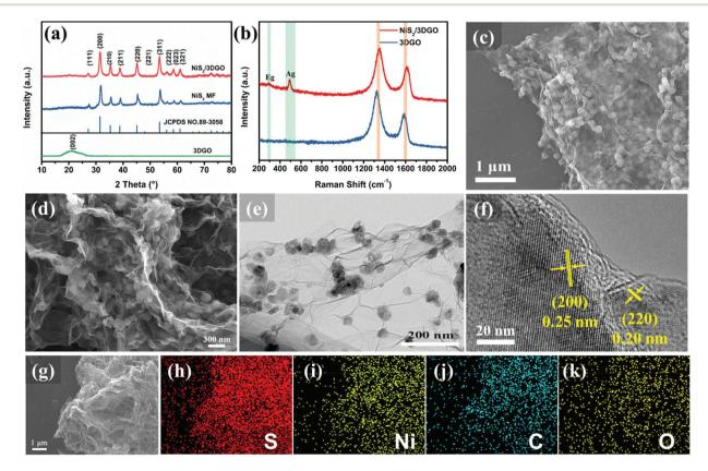
Fig. 2 (a) XRD comparison of NiS<sub>2</sub>/3DGO, NiS<sub>2</sub> MF and 3DGO; (b) Raman spectrum of NiS<sub>2</sub>/3DGO and 3DGO; (c and d) Representative SEM images of NiS<sub>2</sub>/3DGO; (e and f) TEM and HRTEM images of NiS<sub>2</sub>/3DGO; (g-k) SEM images and corresponding elemental mapping analysis of NiS<sub>2</sub>/3DGO.
