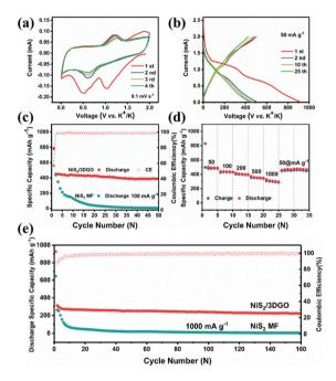
Fig. 4 (a) CV test result for the initial four cycles of NiS<sub>2</sub>/3DGO at 0.1 mV s<sup>-1</sup>. (b) Representative galvanostatic discharge/charge curves of  $NiS_2/3DGO$  at 50 mA  $g^{-1}$ . (c) Cycling performance of  $NiS_2/3DGO$  and NiS<sub>2</sub> MF at 100 mA g<sup>-1</sup>. (d) Rate performance of NiS<sub>2</sub>/3DGO at a different density. (e) Long-term cycling stability of NiS2/3DGO at  $1000 \text{ mA g}^{-1}$
