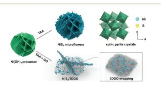
Fig. 1 Schematic illustration of the synthesis process for NiS<sub>2</sub>/3DGO and NiS<sub>2</sub> MF and the proposed stabilizing effects of 3DGO on the NiS<sub>2</sub> electrode.
