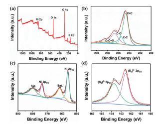
Fig. 3 (a) The XPS survey spectra of NiS<sub>2</sub>/3DGO; (b) C 1s; (c) Ni 2p;
