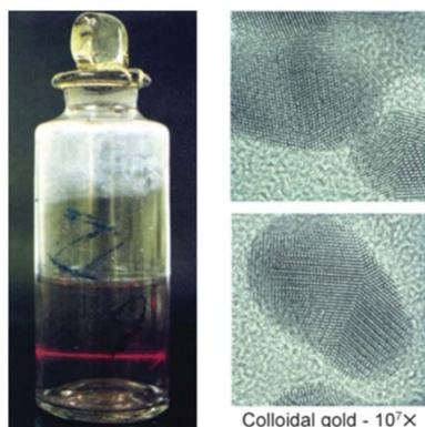
Fig. 5 Faraday's colloidal gold showing the Tyndall effect and transmission electron micrograph of the GNPs.<sup>116</sup> This figure has been adapted/reproduced from ref. 116 with permission from John Wiley and Sons, copyright 2007.
