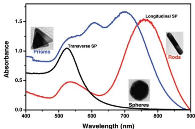
Fig. 4 Localized surface plasmon resonance absorption band for gold spherical nanoparticles (black line), nanorods (red line) and prisms (blue line).<sup>80</sup> This figure has been adapted/reproduced from ref. 80 with permission from RSC, copyright 2015.
