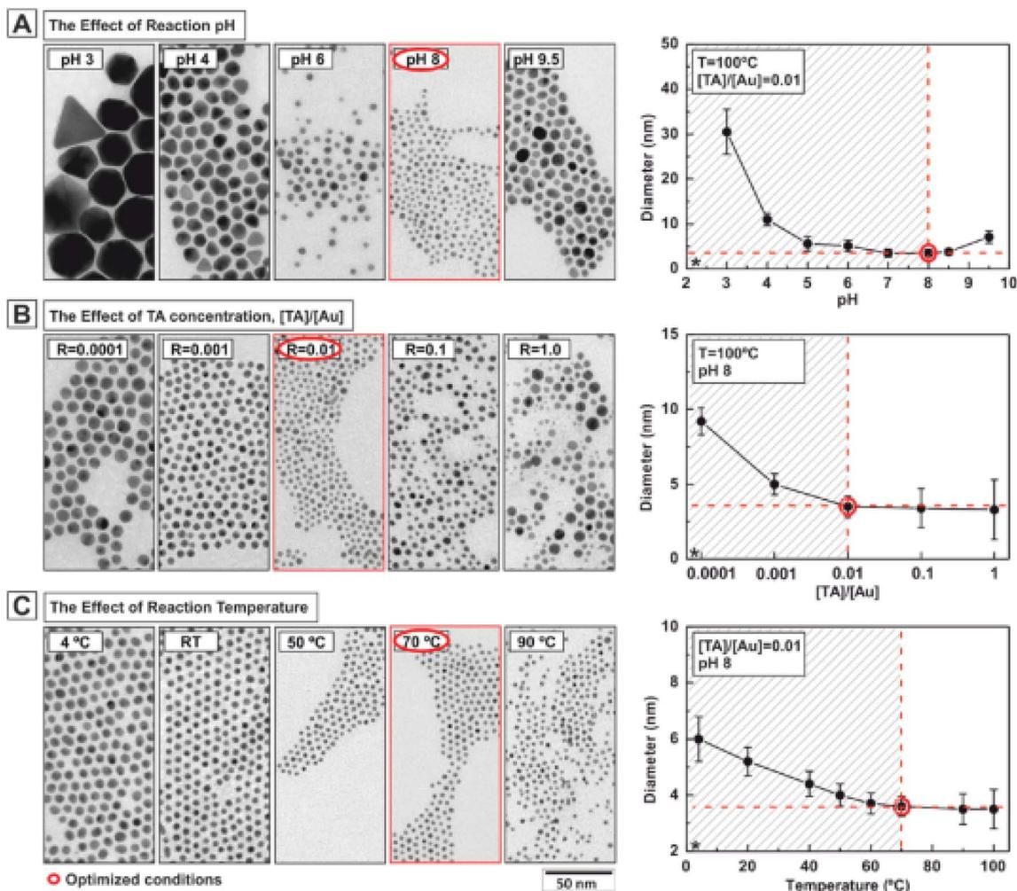
Fig. 6 Effect of reaction parameters on the characteristics of gold nanoparticles. Effect of (A) pH, (B) tannic acid concentration and (C) temperature on the size of gold nanoparticles.<sup>119</sup> This figure has been adapted/reproduced from ref. 119 with permission from the American Chemical Society, copyright 2016.
