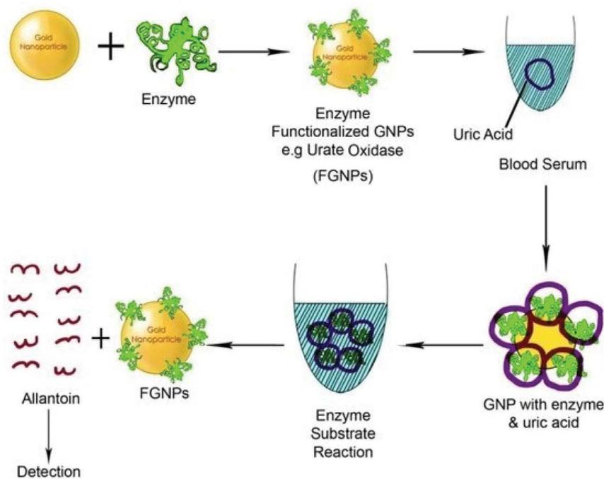
Fig. 12 Schematic diagram of a functionalized gold biosensor to detect serum protein.<sup>254</sup> This figure has been adapted/reproduced from ref. 254.
