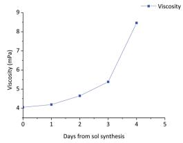
Fig. 4 Variation of the viscosity of the 0.9Nd<sup>3+</sup>-80SiO<sub>2</sub>:20LaF<sub>3</sub> particulate sol as a function of aging time up to the gelification point.
