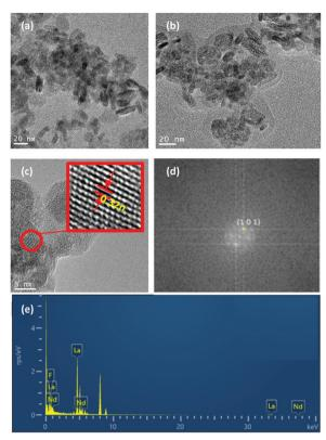
Fig. 3 HRTEM images of (a)  $Nd^{3+}$  –  $LaF_3$  – 0.04 M powder and (b)  $Nd^{3+}$  –  $LaF_3$ -PVP(10)-0.25 M powder (c) single nanocrystal showing a lattice spacing of 0.325 nm for sample  $0.9Nd^{3+}$  – LaF<sub>3</sub> – 0.25 M–PVP(10) (d) FFT pattern corresponding to (c) and (e) EDX analysis of the region.
