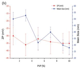
Fig. 1 (a) Variation of the ZP (Mv) of LaF $_3$ -0.04 M nanoparticle suspensions as a function of pH and (b) variation of the zeta potential and particle size of LaF $_3$ -0.04 M nanoparticle suspensions at pH = 7 as a function of PVP wt%.
