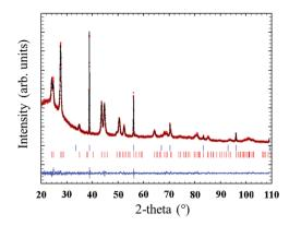
**Fig. 7** Observed (red circles), calculated (continuous black line) and difference (continuous blue line) X-ray diffraction profiles of  $0.9 \text{Nd}^{3+} - 80 \text{SiO}_2: 20 \text{LaF}_3$  particulate sol powders treated at 450 °C for 6 h with 5% NaF as internal standard. The Bragg peaks of NaF and LaF $_3$  are indicated by top and bottom vertical bars, respectively.
