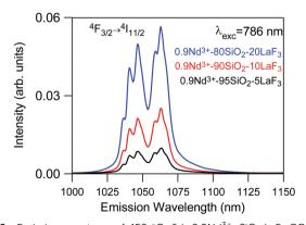
Fig. 10 Emission spectrum of 450 °C-6 h 0.9Nd<sup>3+</sup>-SiO<sub>2</sub>:LaF<sub>3</sub> GCs with three different crystalline fractions 5% (black), 10% (red) and 20% (blue) obtained under 786 nm excitation
