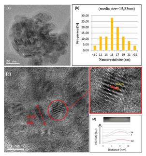
Fig. 6 (a) HRTEM image of  $0.9 \text{Nd}^{3+} - \text{LaF}_3$  nanoparticles in the  $0.9 \text{Nd}^{3+} - 80 \text{SiO}_2$ :20LaF $_3$  sol. (b) Distribution of nanocrystal size of the nanoparticles in the sol. (e) EDX of the corresponding  $0.9 \text{Nd}^{3+} - \text{LaF}_3$  nanoparticle and its scanning lines.
