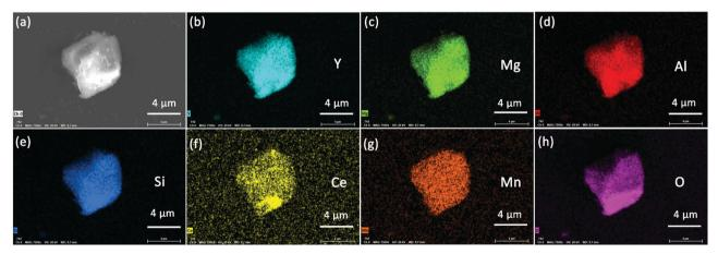
Fig. 4 SEM and element mapping images of YMAS:0.06Ce<sup>3+</sup>,0.20Mn<sup>2+</sup>
