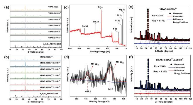
Fig. 1 XRD patterns of YMAS:xCe<sup>3+</sup> (x = 0 - 0.10) (a) and YMAS:0.06Ce<sup>3+</sup>,yMn<sup>2+</sup> (y = 0 - 0.25) (b) with the standard of Y<sub>3</sub>Al<sub>5</sub>O<sub>12</sub> (PDF #88-2048). The XPS survey spectrum (c) and high-revolution spectrum (d) of YMAS:0.06Ce<sup>3+</sup>,0.25Mn<sup>2+</sup>. Rietveld refinement results of YMAS:0.06Ce<sup>3+</sup> (e) and YMAS:0.06Ce<sup>3+</sup>,0.05Mn<sup>2+</sup> (f).
