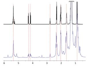
Fig. 1 Proton NMR spectra in CDCl<sub>3</sub> for isolated peanut oil (upper spectrum) and hexanes-extractable material (lower spectrum) from peanut shells used to prepare PS<sub>x</sub>. The spectrum for isolated peanut oil is reprinted from E. G. Silveira Jr, et al., Potential of Virginia-type peanut (Arachis hypogaea L.) as feedstock for biodiesel production, Ind. Crops Prod., 89, 451, © 2016, with permission from Elsevier.
