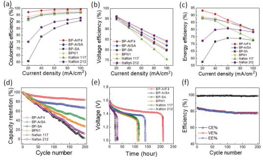
Fig. 2 VRFB single cell performance. (a) CE for PEMs at a current density from 20 to 100 mA cm<sup>-2</sup>, (b) VE for PEMs at a current density from 20 to 100 mA cm<sup>-2</sup>, (c) EE for PEMs at a current density from 20 to 100 mA cm<sup>-2</sup>, (d) capacity retention for IEMs at 100 mA cm<sup>-2</sup>, (e) self-discharge curves of PEMs, and (f) cycling stability of VRFB with the BP-ArF4 membrane at 100 mA cm<sup>-2</sup>.
