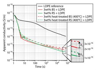
Fig. 3 Apparent conductivity at 60  $^{\circ}\text{C}$  with an electric field of 30 kV mm $^{-1}$ for ZnO LDPE composites containing 3 wt% unmodified or heat-treated (400 °C) particles in the shape of rods or balls. The reproducibility of measurements on the composites containing heat-treated particles is shown in Fig. S3 (ESI†).
