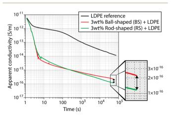
Fig. 2 Apparent conductivity of composites containing 3 wt% ball- or rod-shaped particles and of pristine LDPE at 30 kV mm<sup>-1</sup> at 60 °C. Several measurements up to 2 days were made independently on separately prepared samples, see Fig. S2 (ESI†)
