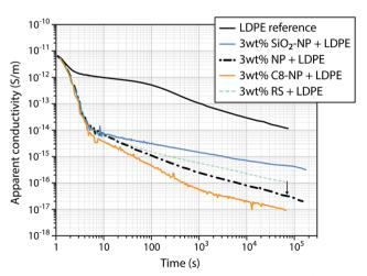
Fig. 7 The apparent conductivity at 60  $^{\circ}$ C and 30 kV mm $^{-1}$  for LDPE composites containing 3 wt% ZnO nanoparticles.
