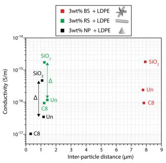
Fig. 9 Composite conductivity after 15 h of polarization as a function of the average inter-particle distance. Composites with unmodified particles are denoted 'Un'.
