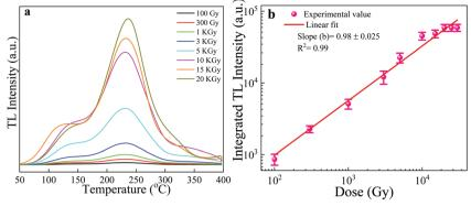
Fig. 9 TL glow curves of the NaGdF<sub>4</sub>:3% Tb<sup>3+</sup> phosphor irradiated with various doses (100 Gy to 20 kGy) of gamma rays from a  $^{60}$ Co source (a). Linear TL response of the NaGdF<sub>4</sub>:3% Tb<sup>3+</sup> phosphor as a function of irradiation dose (b)
