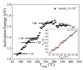
**Fig. 12** Activation energy (eV) vs.  $T_{\text{stop}}$  (°C) plot resulting from the IR method after the  $T_{\text{m}}$ – $T_{\text{stop}}$  procedure for the NaGdF<sub>4</sub>:3% Tb<sup>3+</sup> phosphor irradiated with gamma radiation of 10 kGy doses. A plot of  $T_{\text{m}}$  as a function of  $T_{\text{stop}}$  for the NaGdF<sub>4</sub>:3% Tb<sup>3+</sup> phosphor as an inset image.
