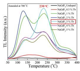
Fig. 8 Thermoluminescence glow curve optimization of the NaGdF<sub>4</sub>:x% Tb<sup>3+</sup> (x = 0, 0.5, 1, 2, 3, 4, 5) phosphor annealed at 700 °C, irradiated at a gamma dose of 1 kGy. NaGdF<sub>4</sub>:3% Tb<sup>3+</sup> showed the most suitable glow curve at 230 °C.
