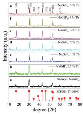
Fig. 1 The XRD patterns of β-NaGdF<sub>4</sub>:x% Tb<sup>3+</sup> (x = 0, 0.5, 1, 2, 3, 4, 5) (a-g) and the standard data of the hexagonal β-NaGdF<sub>4</sub> (JCPDS- 27-0699) as a reference
