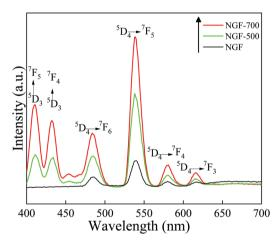
**Fig. 7** The photoluminescence emission spectra of the pristine NaGdF<sub>4</sub>:3% Tb<sup>3+</sup> phosphor crystals and NaGdF<sub>4</sub>:3% Tb<sup>3+</sup> phosphor annealed at 500 °C and 700 °C, monitored at  $\lambda_{\rm ex}$  = 228 nm. The emission intensity increased at higher annealing temperatures.
