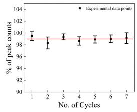
Fig. 11 Reproducibility curve of the NaGdF<sub>4</sub>:3% Tb<sup>3+</sup> phosphor irradiated with 10 kGy gamma rays.
