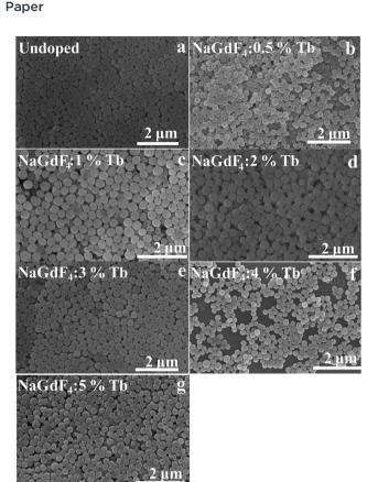
Fig. 2 The FESEM images of  $\beta$ -NaGdF<sub>4</sub>:x% Tb<sup>3+</sup> crystals (x = 0, 0.5, 1, 2, 3, 4, 5) (a–g) showing the spherical morphology of the as-prepared  $\beta$ -NaGdF<sub>4</sub>:x% Tb<sup>3+</sup> phosphors.
