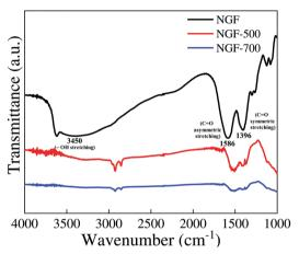
Fig. 5 FTIR spectra of the as-prepared (NGF), 500 °C (NGF-500) and 700 °C (NGF-700) annealed NaGdF<sub>4</sub>:3% Tb<sup>3+</sup> phosphor crystals.
