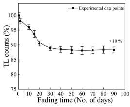
Fig. 10 Fading curve of the NaGdF<sub>4</sub>:3% Tb<sup>3+</sup> phosphor at a 10 kGy dose of gamma-ray irradiation at different time intervals, up to 90 days.
