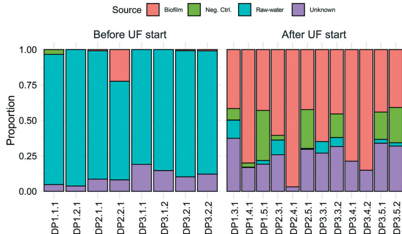
Fig. 3 Identification of the origin of bacteria in the DPs using SourceTracker. Colored bars show the estimated proportion of bacteria from biofilm, negative control (neg. ctrl), raw-water or unknown sources. Samples are ordered in rows and named by their DP number, followed by sampling time and replicate. Each bar is one biological replicate.
