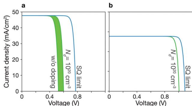
Fig. 7 Current–voltage simulation.  $J$ – $V$  curves for CZTSe (a) and AZTSe (b) solar cells based on the properties of the bulk absorber materials and not including interfacial processes. Green lines represent the TLCs with various doping concentrations up to  $10^{20}$   $\text{cm}^{-3}$ . The SQ limit is shown in the blue curve.
