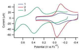
Fig. 3 Cyclic voltammograms of 1, 2, and 3 immobilized on nanoITO substrates in  $0.1 \text{ M } n\text{Bu}_4\text{PF}_6$  in CH $_3\text{CN}$ .
