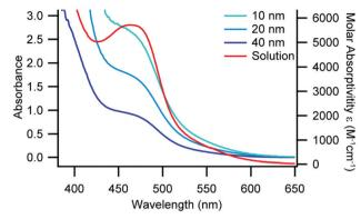
Fig. 1 UV-Vis absorbance of 3 in CH<sub>2</sub>Cl<sub>2</sub> (red, right axis) and immobilized in AAO pores of various pore size (blue traces, left axis), constant path length.
