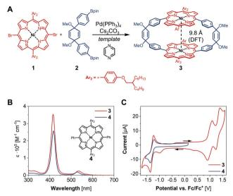
Fig. 2 (A) Synthesis of **3**, Ni–Ni distance obtained by DFT (B3LYP/6-31G(d)). (B) UV/vis absorption spectrum (CH $_2$ Cl $_2$ ) of **3** compared to the reference compound **4**. (C) Cyclic voltammogram of 1 mM **3** and 1 mM complex **4** in CH $_2$ Cl $_2$  with 0.1 M [ $^7$ Bu $_4$ N][PF $_6$ ] at 100 mV s $^{-1}$ .
