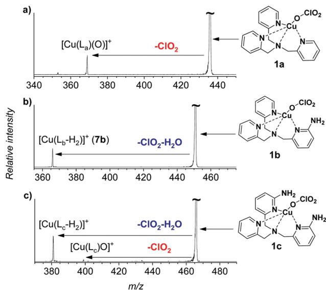
**Fig. 1** Collision induced dissociation spectra of  $[(\text{Ligand})\text{Cu}(\text{ClO}_3)]^+$  complexes with xenon as the collision gas ( $P_{\text{Xe}} = 0.1$  mTorr) at a collision energy of  $\sim 4.2$  eV in the centre of mass frame.
