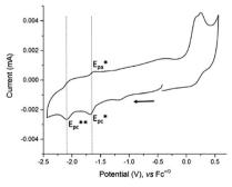
Fig. 2 Cyclic voltammogram of 4, concentration 0.3 mM at a stationary glassy carbon electrode (3 mm diameter) in DMF + 0.1 M  $\rm NEt_4ClO_4$ . Scan rate 100 mV s<sup>-1</sup>.
