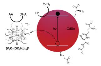
Fig. 1 Illustration of the general photocatalytic scheme. Upon excitation by visible light, the electron reduces protons at the surface of the QD, while the hole is extracted by a POV-alkoxide cluster. Ascorbic acid (AA) is used to regenerate the reduced form of the cluster in solution. Capping ligands were chosen to promote solubility in aqueous solutions, and include cysteine (top), glutathione (middle), and 3-mercaptopropionic acid (bottom). DHA indicates dehydroascorbic acid.
