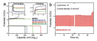
Fig. 4 Rechargeable ZAB performance: (a) capacity plots at 5 mA cm<sup>-2</sup> with different BPMC cathode materials and (b) cyclic stability test of BPMC/ NCNT-10 cathode
