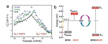
Fig. 2 (a) Mott Schottky plots of BPMC/NCNT-10 at three different frequencies. (b) Schematic diagram of  $E_{\rm fb}$  alignment of BPMC, NCNT and BPMC/NCNT-10 with respect to standard  ${\rm O_2}$  electrolysis potential in alkaline medium.
