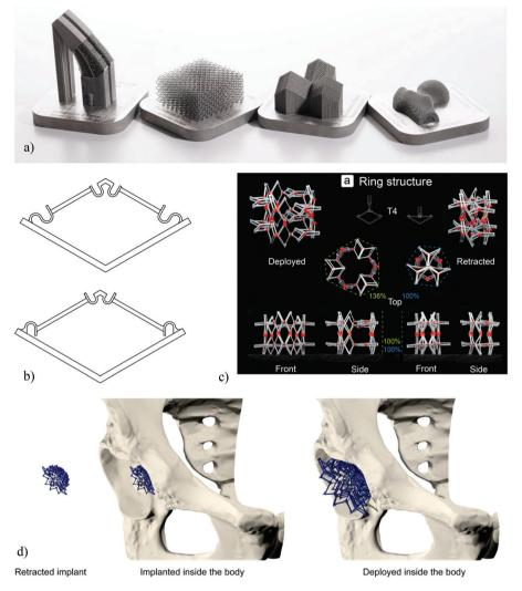
Fig. 1 (a) A number of AM orthopaedic implants (reprinted from ref. 46 with permission from Elsevier, Copyright 2018). (b) The basic bi-stable elements used for the design of multi-stable deployable implants.<sup>38</sup> (c) A deployable implant made through an arrangement of bi-stable implants.<sup>38</sup> (d) A schematic demonstration of the concept of deployable implants.<sup>38</sup>
