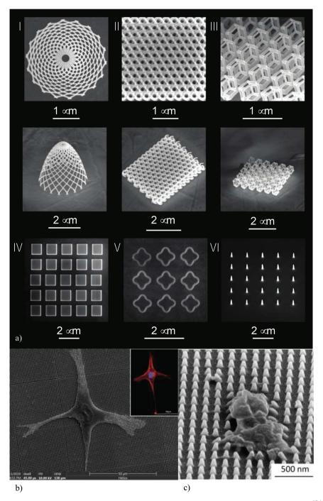
Fig. 5 (a) Some examples of the nanofeatures created on the surface of origami-based meta-biomaterials using EBID.<sup>104</sup> (b) The response of preosteoblast to nanopatterned surfaces. (c) *Staphylococcus aureus* can be killed by nanopatterns.<sup>95</sup>
