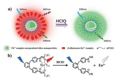
Fig. 6 Design concept of a ratiometric luminescent probe based on crow-like dual-emissive silica nanoparticles modified by Tb<sup>3+</sup> and Eu<sup>3+</sup> complexes (a), and the luminescence quenching mechanism of a  $\beta$ -diketonate-Eu<sup>3+</sup> complex by HClO (b). Reprinted with permission from ref. 115. Copyright 2017, Royal Society of Chemistry.
