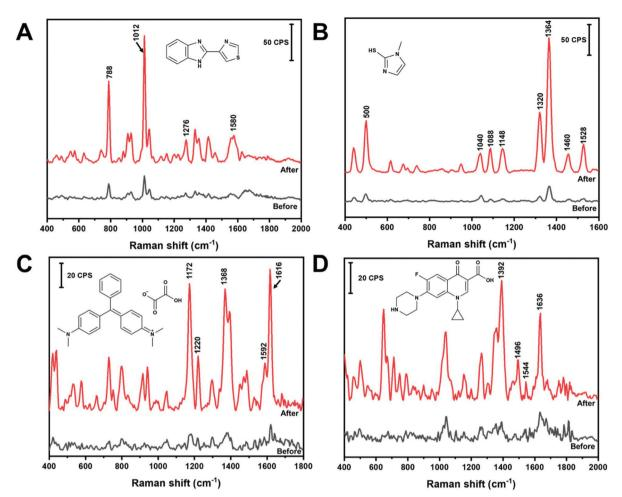
Fig. 6 (A) 5 µM thiabendazole in 0.1 M HCl, (B) 1 µM methimazole in water, (C) 0.5 µM malachite green in water and (D) 5 µM ciprofloxacin in 0.1 M HCl using a colloidal AuNS HR100 substrate before and after the addition of NaCl (200 mM).
