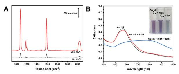
Fig. 5 (A) SERS spectra of MBN using AuNS HR100 before and after salt addition. (B) UV-Vis spectra showing the extinction of AuNS HR100, after the addition of MBN and after the addition of MBN and NaCl.
