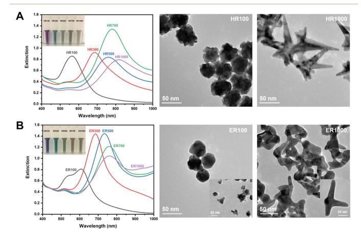
Fig. 2 Extinction spectra of (A) HEPES and (B) EPPS buffers. The inset images show the colour of the AuNS solutions at the given ratios. TEM images correspond to AuNS at *R* 100 and 1000.
