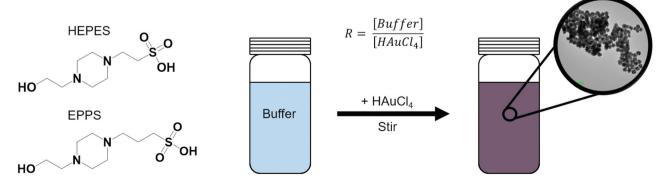
Fig. 1 Schematic of AuNS synthesis using Good's buffers (HEPES and EPPS).
