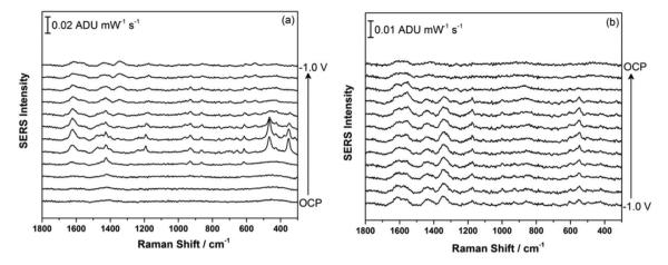
Fig. 2 (a) EC-SERS signal for THC on the AgNP-modified SPE at OCP, and then from 0.0 to -1.0 V in 100 mV increments. (b) EC-SERS signal stepping back from -1.0 V to 0.0 V in 100 mV increments, and finally at OCP measured after the potential stepping. Spectra measured at 780 nm, 80 mW, 30 seconds.
