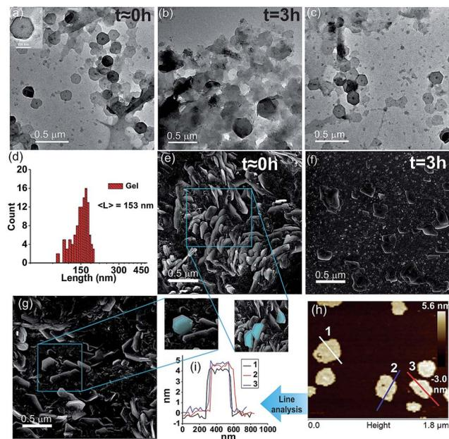
**Fig. 2** TEM images of (a) **C18A-Fc-NMe<sub>2</sub>** for  $t \approx 0$  h (inset: enlarged view), (b)  $t = 3$  h sol, and (c) refueled gel (4 mM **Fc-NMe<sub>2</sub>**). (d) Histogram of hexagon dimensions from the TEM results at  $t \approx 0$  h. SEM images (e) at  $t \approx 0$  h with blue traces showing the hexagonal structures, (f)  $t = 3$  h sol, (g) refueled gel (5 min), and (h) AFM image at  $t \approx 0$  h and (i) the corresponding height profiles.
