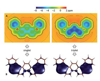
Fig. 7 (A) NICS(1.5) maps (CAM-B3LYP/6-311++G(d,p)) and (B) RAS(4,4)-SF/cc-pVTZ odd-electron density (0.008 a.u. isovalue) calculated for the substituent-free DIPh ring system in the singlet (left) and triplet (right) states.
