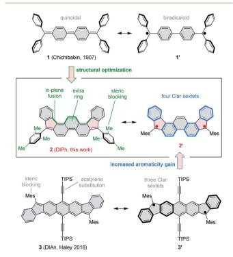
Scheme 1 5,10-Dimesityldiindeno[1,2-a:2',1'-i]phenanthrene (2) and its structural relationship to Chichibabin's hydrocarbon (1) and Haley's diindenoanthracene (3). Mes = mesityl, TIPS = tri(isopropyl)silyl.
