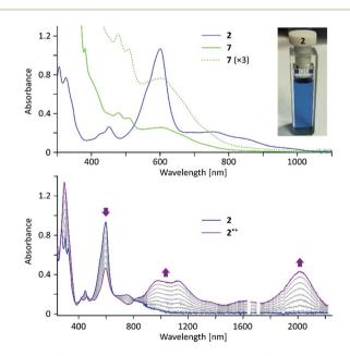
Fig. 2 (Top) Electronic absorption spectrum of 2 (dichloromethane,  $ca. 2 \times 10^{-5}$  M, blue trace) and 7 (dichloromethane, green traces). The photo shows the appearance of 2 in a dichloromethane solution. (Bottom) Formation of the radical cation  $2^{*+}$  (purple) upon oxidation with magic blue. Intermediate titration stages are shown in gray.
