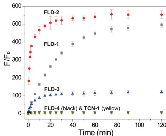
Fig. 4 Fluorescence turn on of **FLD-1** (gray), **FLD-2** (red), **FLD-3** (blue), **FLD-4** (black), and **TCN-1** (dark yellow) (10 μM) in PBS (pH 7.4, 10 mM) containing Cys (100 μM). λ<sub>ex</sub> = 490 nm for **FLD-1**, 2, 4, and **TCN-1**, λ<sub>ex</sub> = 454 nm for **FLD-3**, λ<sub>em</sub> = 500–650 nm, and slit width = 0.3 nm. The experiments were performed in triplicate. The results are expressed as mean ± SD (n = 3).
