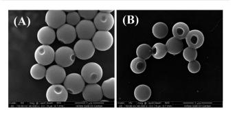
Fig. 2 SEM images of nanobowls formed from (A) PHAzoMA $_{29}$  and (B) PHAzoMA $_{116}$ .
