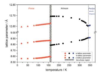
Fig. 4 Temperature dependent lattice parameters of MAPbl $_3$  received from Le Bail refinement of synchrotron XRD pattern. Lattice parameters of orthorhombic, tetragonal and cubic phase are shown. For a better comparability, the pseudo tetragonal a- and c-lattice parameters are used in the high temperature cubic (Pm3m) modification at the phase transition to the lower temperature tetragonal phase.
