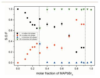
Fig. 3 Site occupancy factors in dependence of educt molar fraction of MAPb( $I_{1-x}Br_x$ ) $_3$  received from Rietveld refinement of XRD powder pattern. Occupancy factors of iodine rich and bromine rich phases in single phase and miscibility gap are shown. For a better comparability, the two phase region is separated by horizontal dotted lines.
