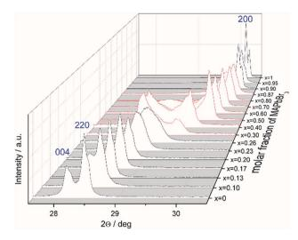
Fig. 1 Powder pattern of selected compositions of the MAPb( $I_{1-x}Br_x$ )<sub>3</sub> solid solution: evolution of the 220 and 004 Bragg peaks of MAPbI<sub>3</sub> with increasing degree of substitution. The change from iodine rich phase towards the 200 Bragg peak of the bromine rich phase is shown (single phase region in black, two-phase region in red).
