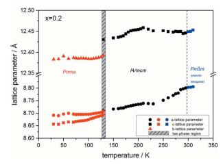
Fig. 6 Temperature dependent lattice parameters of MAPb( $I_{0.8}$ Br $_{0.2}$ ) $_3$  solid solution received from Le Bail refinement of synchrotron XRD pattern. Lattice parameters of orthorhombic, tetragonal and cubic phase are shown. For a better comparability, the pseudo tetragonal a-and c-lattice parameters are used in the high temperature cubic (Pm3m) modification at the phase transition to the lower temperature tetragonal phase.
