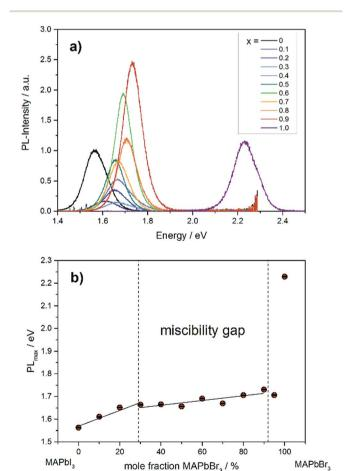
Fig. 9 (a) Photoluminescence spectra of different  $MAPb(I_{1-x}Br_x)_3$  mixed crystals. (b) Dependence of  $PL_{max}$  on the chemical composition in  $MAPb(I_{1-x}Br_x)_3$  solid solutions.
