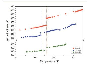
Fig. 7 Temperature dependence of the unit cell volume for MAPbI<sub>3</sub>, MAPbBr<sub>3</sub> and MAPb( $I_{1-x}$ Br<sub>x</sub>)<sub>3</sub> solid solutions with x = 0.20.
