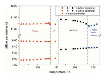
Fig. 5 Temperature dependent lattice parameters of pure  $MAPbBr_3$  received from Le Bail refinement of synchrotron XRD pattern. Lattice parameters of orthorhombic, tetragonal and cubic phase are shown. For a better comparability, the pseudo tetragonal a- and c-lattice parameters are used in the high temperature cubic (Pm3m) modification at the phase transition to the lower temperature tetragonal phase. In addition an incommensurate phase (IC) is present.
