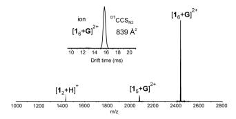
Fig. 1 (+)ESI-MS spectrum of 1 (60  $\mu$ M) and tris(bipyridine)ruthenium( $_{\rm II}$ ) (G) with 6:1 ratio measured from acetone/DCM mixture. Inset showing IMS arrival time distribution (ATD) for  $[1_6+G]^{2+}$  ion.
