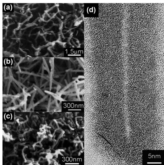
Fig. 11 SEM images of CNT brushes grown on (a) polycarbonate and (b and c) Teflon substrates with (a) cobalt naphthenate and (b and c)  $\text{Co}_9\text{S}_8$  as the catalysts. (d) HRTEM image of the MWNT grown in (b). Reproduced from ref. 35, with permission from Wiley, 2003.
