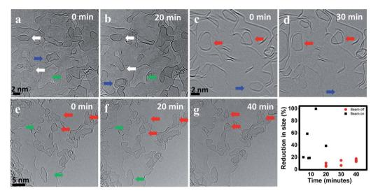
Fig. 5 BF-TEM images of the same region before and after 20 minutes of heating at 900 °C (a, b), (c, d) and (e-q) at 1200 °C. The graph shows the percentage of reduction in size of selected graphene flakes during heating with the electron beam on (black) and off (red).
