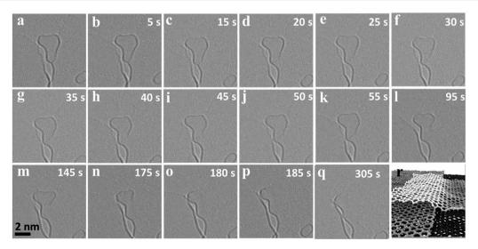
Fig. 2 (a-q) Slow merging of a nanoflake with an edge in the layer underneath during heating at 1200 °C, the time interval is shown as label in each micrograph. (r) shows a MD simulation of pinning of a flake (dimensions of approx.  $5.5 \times 5 \text{ nm}^2$ , hydrogen-free edges) to the step edge below at 1500 K.
