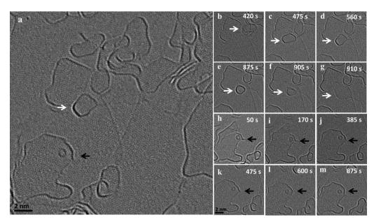
Fig. 3 (a) HRTEM image of an area in which shrinkage of a migrating flake (indicated by the white arrow) and growth of a larger flake (indicated by black arrow) has been observed simultaneously. (b-g) shows the mass loss during migration of the flake and (h-m) the growth of the large flake by extending the edge.
