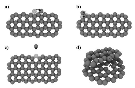
Fig. 6 NEB determined activation energies  $E_A$  for different processes: (a) edge diffusion of an ad-atom ( $E_A = 0.58$  eV), (b) 6- to 5-membered ring reconstruction ( $E_A = 1.76$  eV), (c) atom removal from a zig-zag edge ( $E_A = 9.17$  eV), (d) pinning–depinning process with atom transfer from edge to vacancy ( $E_{A,pinning} = 0.015$  eV <  $k_BT$  and  $E_{A,pinning} = 2.47$  eV). For detailed energy profiles see ESI Fig. 2.†
