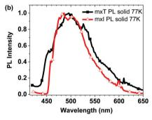
Fig. 3 (a) Absorption spectra and normalized emission spectra in 2-MeTHF at 77 K. (b) Normalized emission spectra in neat solid at 77 K.
