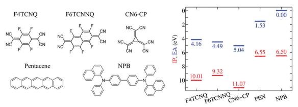
Fig. 1 Molecular structures of the dopant and semiconductor molecules considered in this study. The right panel reports IP and EA for the selected molecules, as obtained from evGW calculations in the gas phase.
