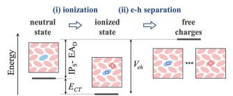
Fig. 5 Illustration of the elementary steps of the p-doping process for a generic molecular semiconductor and of the electronic states involved with their relative energies.  $IP_{Sr}$  EAD and  $E_{CT} = IP_{S} - EAD + V_{eh}$  do all refer to the adiabatically relaxed values. The dopant molecule in the host OSC is depicted in light blue.
