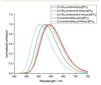
Fig. 13 Normalized emission spectra of  $[Cu(P^P)(N^N)][PF_6]$  complexes in Me-THF at 77 K ( $\lambda_{exc}$  = 410 nm).
