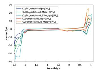
Fig. 9 Cyclic voltamogramms of  $[Cu(P^AP)(N^AN)][PF_6]$  compounds in  $CH_2Cl_2$  at a scan rate of 100 mV s<sup>-1</sup> referenced to internal Fc/Fc<sup>+</sup> = 0 V.
