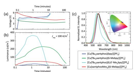
Fig. 14 Time evolution of the (a) voltage and (b) the luminance for a series of LECs driven at an average current density of  $100 \text{ A m}^{-2}$ . (c) Electroluminescence spectra for the same device series with (inset) the corresponding colour coordinates in the CIE 1931 colour space.
