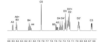
Fig. 6 Aromatic region of the  $^{1}$ H NMR spectrum (500 MHz, acetone- $d_{6}$ ) of [Cu( $^{t}$ Bu<sub>2</sub>xantphos)(6-Mebpy)][PF<sub>6</sub>]. See Scheme 3 for atom labelling.
