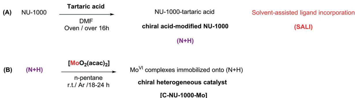
Scheme 1 The preparation steps of (N + H) and [C-NU-1000-Mo] catalyst with the used conditions.
