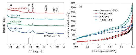
Fig. 1 (a) XRD patterns and (b) N<sub>2</sub> adsorption-desorption isotherms of the as-prepared catalysts and NiO nanoparticles.
