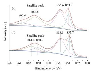
Fig. 3 XPS spectra of Ni 2p<sub>3/2</sub> of (a) NiO(P)-300 and (b) commercial NiO samples.
