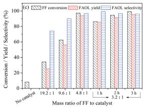
Fig. 4 (a) Effect of reaction temperature and reaction time on CTH of FF to FAOL (1 mmol FF, 0.02 g NiO(P)-300, 5 mL 2-propanol); (b) effect of alcohol as H-donor on CTH of FF to FAOL (1 mmol FF, 0.02 g NiO(P)-300, 5 mL alcohol, 120 °C, 3 h, formation rate calculated from the FAOL yield obtained after 3 h); (c) effect of catalyst dosage on the CTH of FF to FAOL (1 mmol FF, 5 mL 2-propanol, 120 °C, 3 h, mass ratio of FF to catalyst ranging from 19.2 to 3.2).
