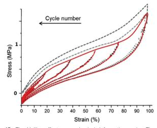
Fig. 13 The Mullins effect on mechanical deformation cycles. The top figure shows repeated cycling to a given deformation followed by repeated cycling to a higher strain, whereas the lower figure shows repeated cycling but with decreasing strains utilised. The dotted curves are the initial cycle. whereas the red curves are the subsequent four cycles. Reproduced from ref. 14 with permission from the Technical University of Denmark (DTU), copyright 2017.
