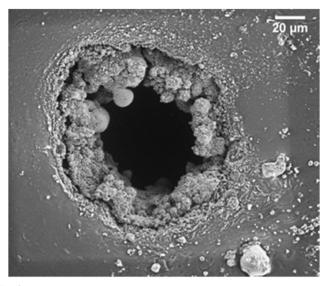
Fig. 8 Breakdown zones of a chloropropyl-functional copolymer crosslinked into elastomers (details of elastomers in article). <sup>36</sup> Reproduced from ref. 14 with permission from the Technical University of Denmark (DTU), copyright 2017.
