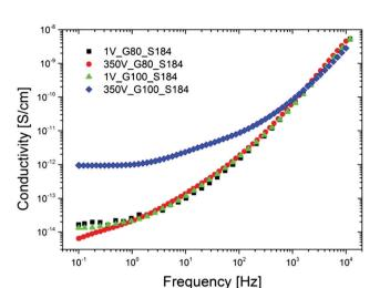
Fig. 7 Illustration of the electrical field dependency of silicone elastomers with high loadings of high-permittivity substances (glycerol). Conductivity of various glycerol–Sylgard 184 composites with 80 phr and 100 phr loading, respectively, at 1 V and 350 V and at room temperature.<sup>29</sup> Reproduced from ref. 29 with permission from the Wiley Periodicals, Inc., copyright 2016.
